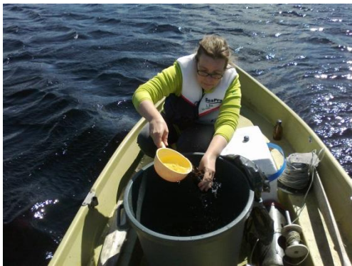
Figure 4.21 - Phytoplankton samples, taken with a Limnos sampler, were pooled in a plastic container, protected from light (see Fig. 2.20), before filling in the sample bottles.
