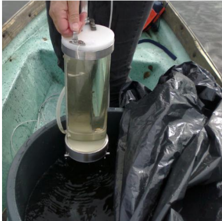
Figure 4.20 - Phytoplankton samples were taken with a Limnos tube sampler to take integrated water samples that represented either euphotic or mixed layers.
