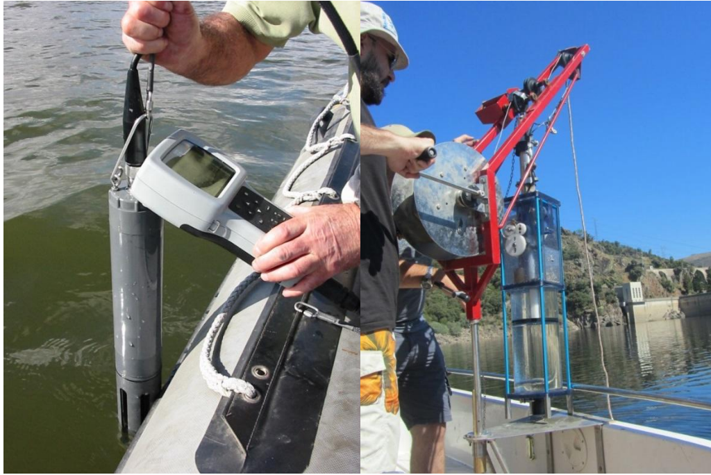
Figure 4.35 - Left, the YSI 6600 probe being lowered in the water, and right, the UWITEC integrated sampler before extracting the sample to the homogenizing container.
