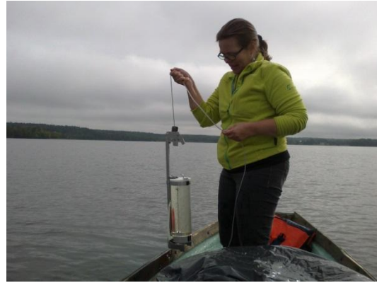
Figure 4.20 - Phytoplankton samples were taken with a Limnos tube sampler to take integrated water samples that represented either euphotic or mixed layers.
